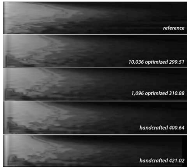
Fig. 8: The computed MPEG-7 spectral envelopes of the compared Black Water Reverb generated settings mapped to grayscale. The numbers behind the settings' names indicate the resulting distance to the reference.
