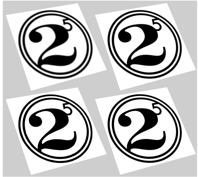
Figure 3: Comparison of techniques: standard trilinear filtering ( 128 \times 128 texels, 21 KB, upper left), our method (same resolution and memory size, lower left), DXT1-compressed trilinear filtered texture ( 256 \times 256 texels, 43 KB, upper right), high-resolution texture ( 1024 \times 1024 texels, 1365 KB, lower right).
