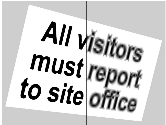
Figure 4: Optimized texture as displayed (left) and before thresholding (right). Note the dots generated to sharpen the corners of the typeface characters.
