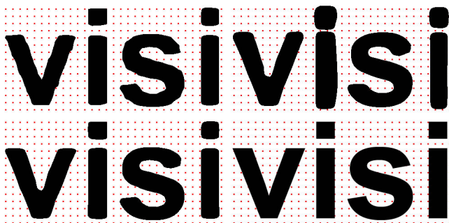
Figure 2: Different distance metrics for the optimization lead to different shapes: square of difference between positions of intersections ( d_l , upper left); square of difference between angles at intersections ( d_a , upper right); the mixed measure d_a + 0.01d_l / (\alpha^2 + 0.01) , which we employ (lower left; for the definition of \alpha see Figure 5). For comparison, the high-resolution bitmap is shown in the lower right.
