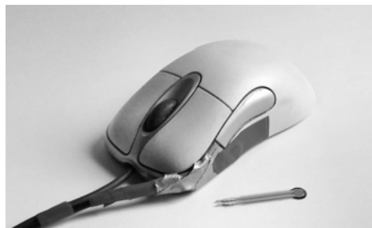
Fig. 1: The pressure-sensitive zoom mode employs a mouse with an attached thumb-operated sensor. A spare pressure sensor is shown in front of the mouse.
