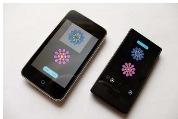
Fig 2: The user interface containing two flower-shaped, procedural buttons, running as native application on the Apple iPod Touch, and as an AJAX Web page on the Microsoft Zune.
