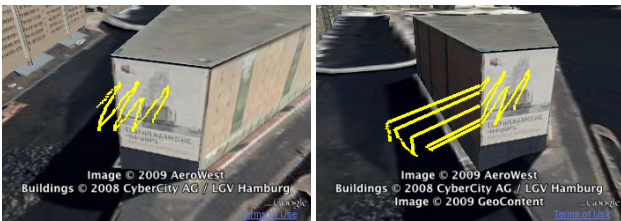
Figure 1: Even though 3D mouse data are available from Google Earth, the results can be surprising when one paints past edges (left: view during painting, right: rotated).
