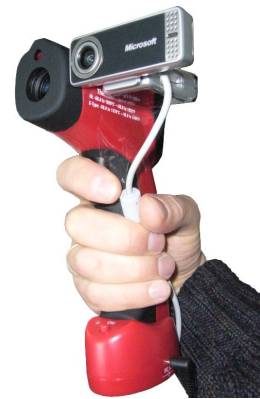
Figure 2: A webcam and an infrared thermometer are coupled to augment each image taken by temperature measurements.
