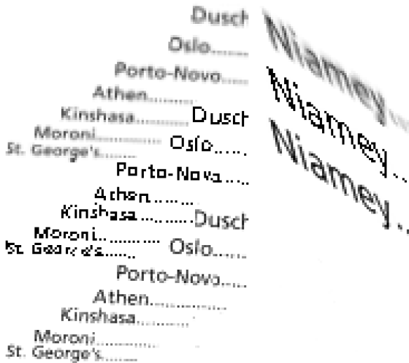
Figure 1: Compared to a standard MIP-mapped texture (upper lines), a 2D font engine delivers highly readable text even at tiny sizes (middle lines: pixelated, lower lines: with font antialiasing). This image uses large pixels deliberately to show the effect. ClearType, the best method, cannot be shown in this grayscale print.
